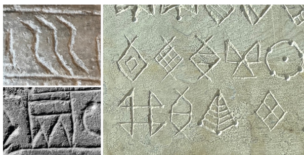
FIG. 47. Thin endings of the strokes. Left: Stone inscriptions A & B. Right: Engraving test on soft limestone
