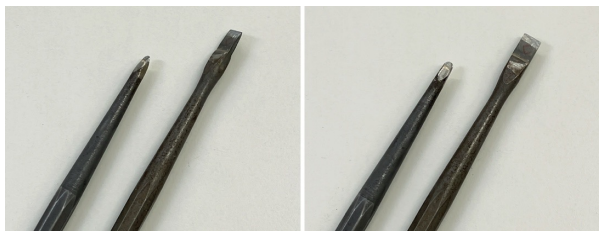
FIG. 46. Tools used for engraving tests. The left one was used for the dots and the right one for the strokes
