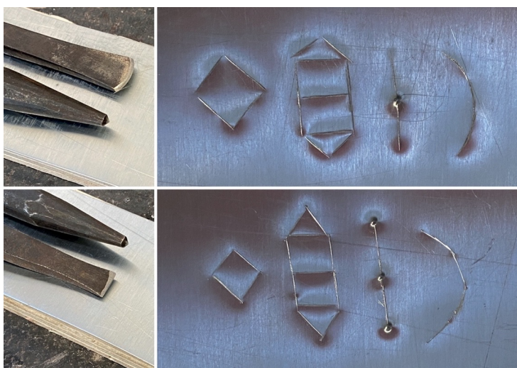
FIG. 37. Experimenting engraving on metal with round and flat tools
