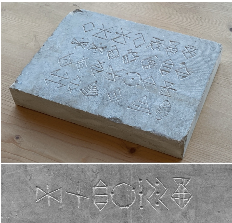
FIG. 45. Top: engraving test on soft limestone. Bottom: engraving test on harder limestone
